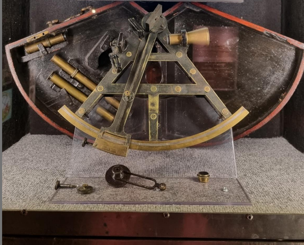
Parts of the Wooden Sextant (Labeled: Mirror, Body, and Telescope)
